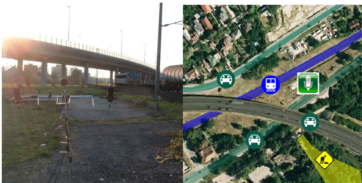
Figure 6 – photo and map of the source selective noise measurement experiment on site
